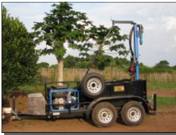
Water drilling rig at Bori.
